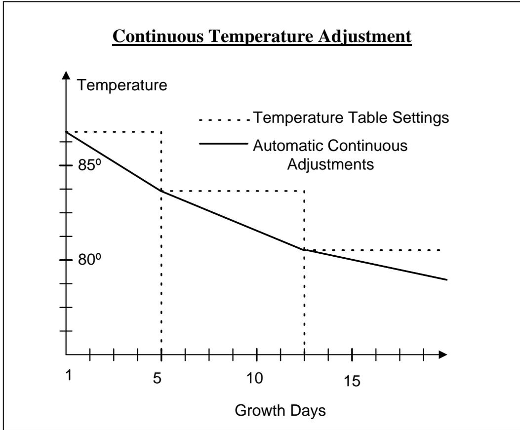
Configuration, menu 91, item 8, “automatic daily temperature adjustment,” controls whether the **AC-2000HP** interpolates between lines of the temperature table and calculates in between set temperatures, or uses only the exact temperatures from the table. Interpolation results in temperature ramping with smooth continuous change. Otherwise, it would jump abruptly at midnight on the growth days programmed in the temperature table.
