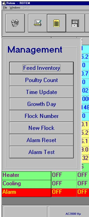
The management menu provides important tools for the poultry producer. These tools record water and feed consumption, how long the heaters have been running, and other important information.
