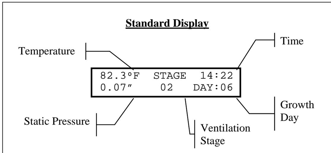
Press the **ESC** key to bring up the control menu. If you press **ESC** again, the standard display will reappear.
