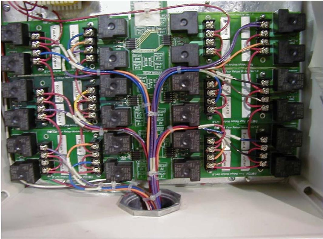
Note that this style wiring makes it easy to replace any relay module when necessary. The main wiring bundle is in the center of the box and does not cover any relay modules.
