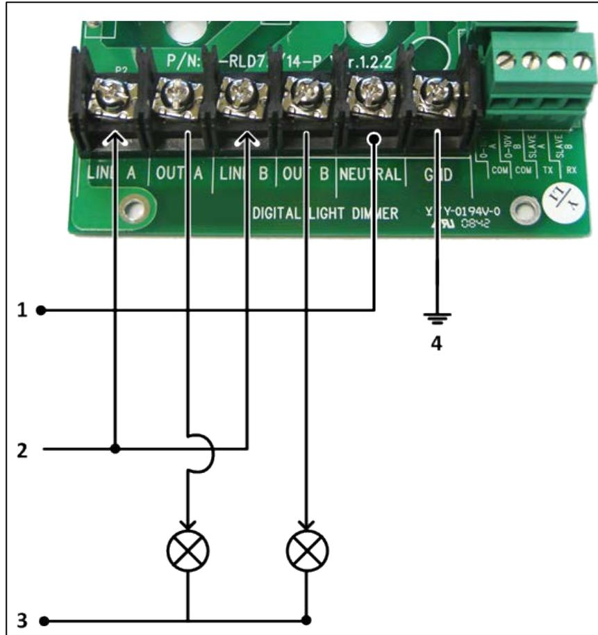
Figure 2: RLED 115V Single Phase Wiring
