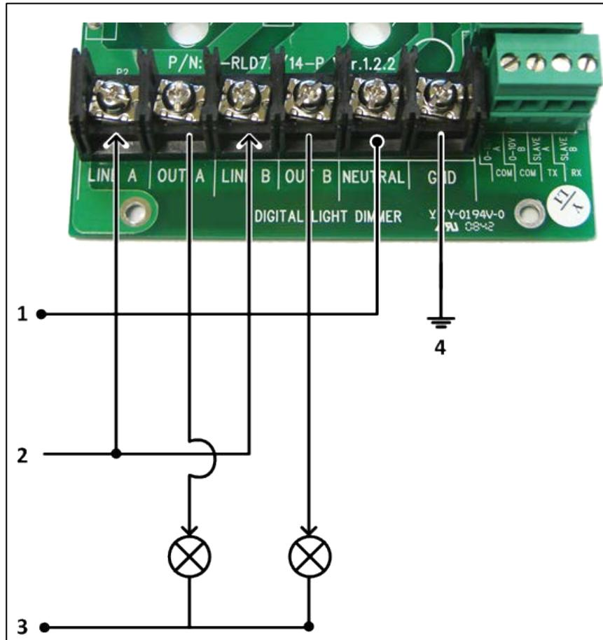
Figure 4: RLED 230V Single Phase Wiring
