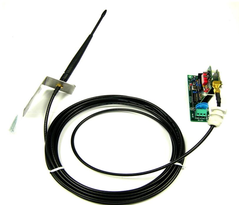
4. Take the antenna and its stand and place on high place where nothing is blocking the LOS (line of sight).
